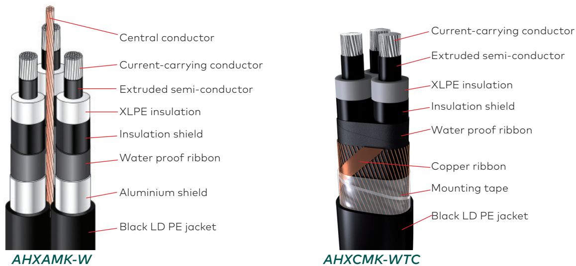
Fig. 1.14. Construction of medium-voltage cables [12].
